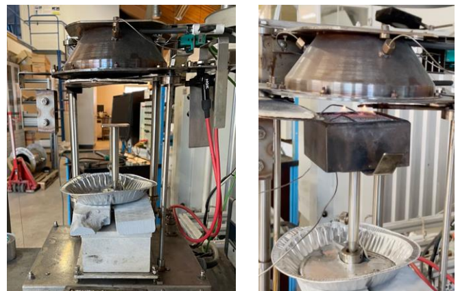
Figure 2. Cone calorimeter test: equipment (left), ongoing test (right)
