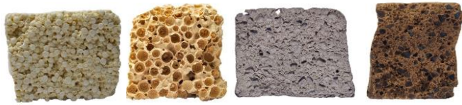
Figure 7. Zoomed photos. From left to right: initial EPS.m, post-heating EPS.m, initial Aero.m, post-heating Aero.
